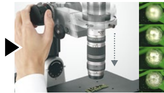
move the lens through the Z range for composition...
